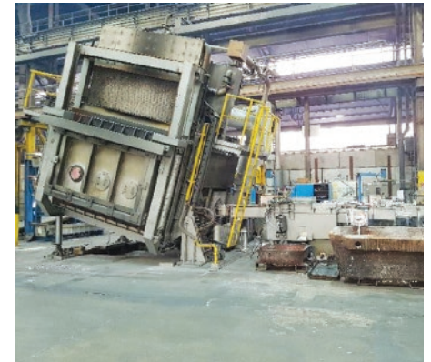
3 Prototype Optifilter installed at the Trimet Aluminium R&D casting pit.
